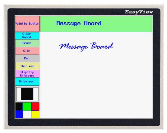
The system keeps LB9020-LB9022 and is used for controlling and combining identification Pen,Brush,Chip,choose or not,LB9030-LB9032 can set the thickness of the pen,LW9006 can set the operation mode,LW9007 can set the thickness of the pen,LW9008 can choose any pen's color from 256 colors. Please refer to Ch12 for detail.
